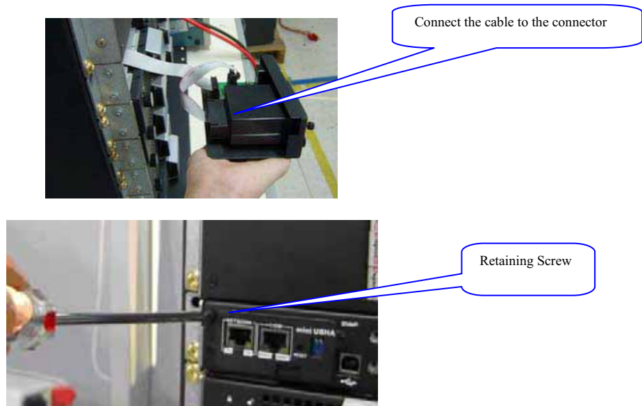
Figure 27 Installing and remove the communication interface module
