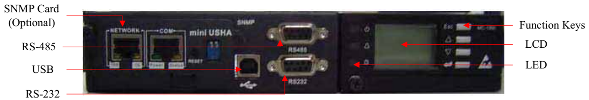
Figure 22 Communications interfaces on the front plate of the controller
