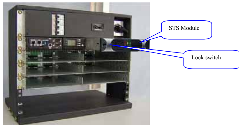
Figure 29 Installing and removing the STS module
